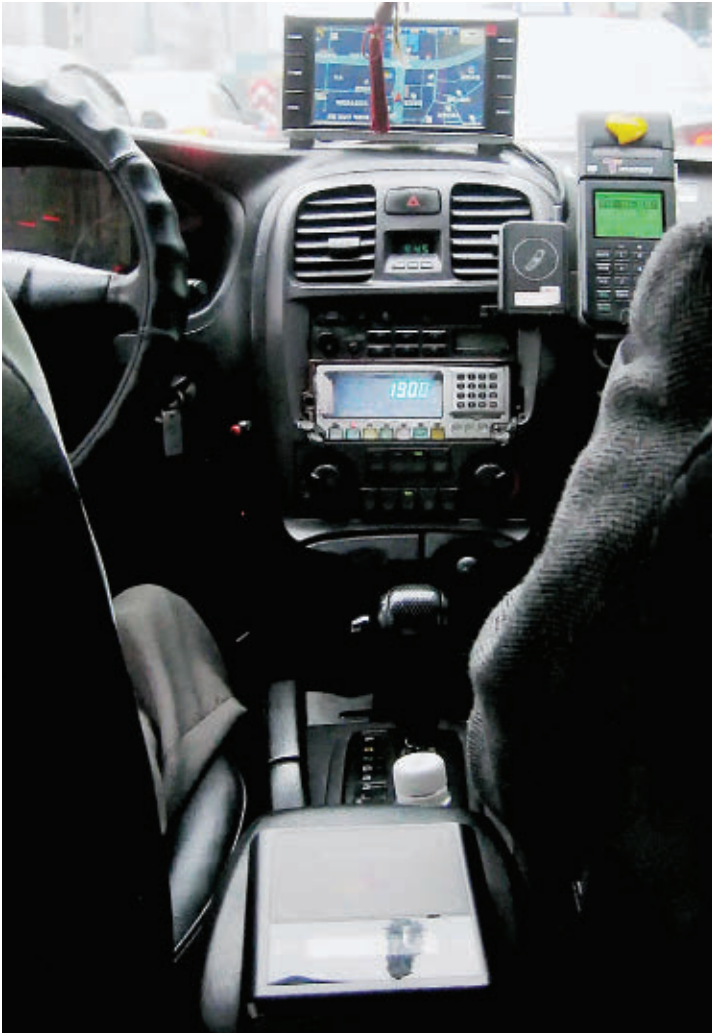
► Figure 1. Taxicab Fare-paying Infrastructure in Korea. (from the center bottom, moving up) The pad where one touches a credit or transportation card with transaction chip; the taxi meter, with calculator keypad for entering the amount of cash payment; the pad where one touches the transaction-enabled cell phone; just to its right, the credit card-reading device for normal credit cards with magnetic stripe, complete with keypad, which I assume is for manual entry or security codes; just above the credit card reader, a printer to provide receipts for any of the payment methods; at the very top center, the navigation system, this time displaying map information instead of a television show. I have skipped over the auto's infrastructure, including radio, tape, and CD player, HVAC controls, shifting controls, and steering wheel, all of which are also visible in this photograph.
