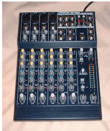
Figure 17.3 Small Behringer 4-line mixer.
