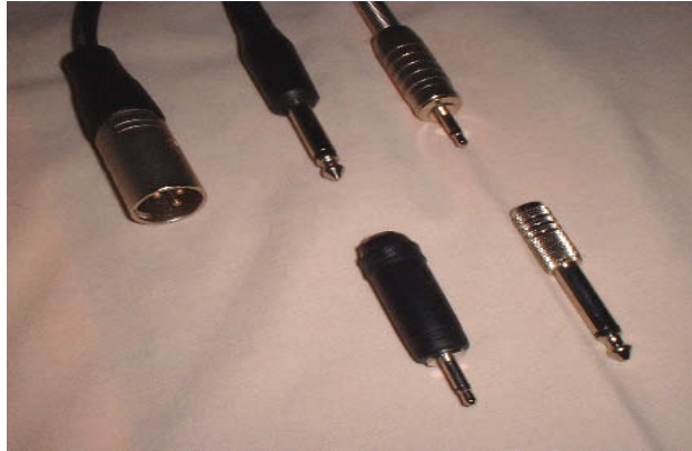
Figure 17.1 Connectors: XLR, one-quarter-inch jack, minijack (one-eighth inch), and converters.
