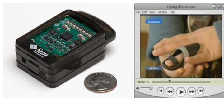
Figure 9. The physiological emotion sensing hardware
