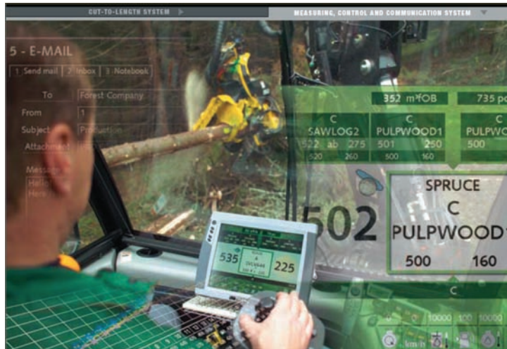
Figure 1. Modern lumberjack cockpit equipped with multiple screens and computers. A view of the Timbermatic 300 system ( www.deere.com/en_US/cfd/forestry/deere_forestry/harvesters/wheel/1070d_flash.html , last accessed 2009.01.31).
