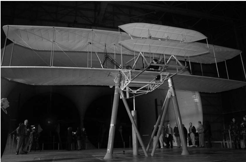
Figure 17.1. Wright 1902 Glider Reproduction Underwent Wind Tunnel Tests at Langley Full-Scale Tunnel.
